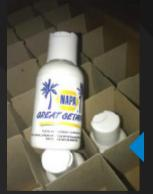
When shipping liquids in a sealed bottle, it is important to apply closures with the correct application torque to ensure that the liner compresses and forms a good seal. **Proper application torque will also help prevent the closures from backing off during vibration.**
