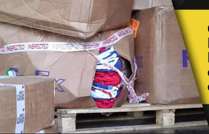
Overfilled boxes will burst; underfilled boxes will collapse, causing damage to the contents.
